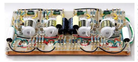
All parts were carefully chosen after massive hours listening tests. High grade audio volume, silver foil capacitors, silver lead resistors, SSW silk silver wires, Ls-41 shield cable, Audio Note custom made output transformers and power transformer.
